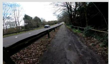
Pinch point due to level differences. Proposed footway widening on the southern side to accommodate a short section of a shared use path. Parapets protecting cyclists and pedestrians from the level difference would need to be upgraded and raised.
