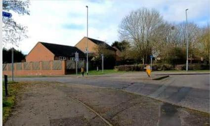
Pinch point created by out of use bus stop. Consider removal of the shelter to accommodate the segregated cycleway.
