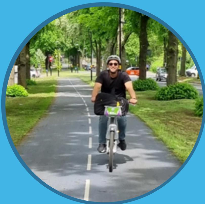
**Segregated cycleway:** a dedicated pathway for bikes that is physically separated from motorised vehicles and pedestrians. These can be one-way or two-way and can be separated by physical barriers such as kerbs or grass verges.
